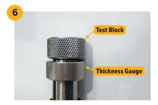
Apply provided Ultrasonic Couplant Lube onto the Block and hold the Probe against the Test Block firmly. The thickness of the Block should now appear on screen within CygLink.
