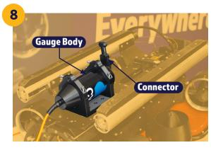
Slide Cygnus Gauge Body onto the ROV Thickness Gauge Mount Adaptor (E). Place the 2 Top Brackets over the Gauge Body and secure with 4 - 9/64" Allen Screws. The Cygnus Gauge Body Connector Faces away from the ROV body.
