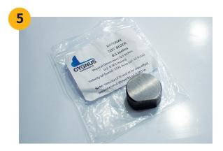
• Before using in the water preform a test with the provided 0.5" Test Block pictured above.
