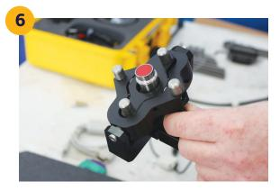
• Push Probe through the Gimbal as shown and tighten the 4 Grub Screws to secure the Probe. Make sure the Probe is seated flush.
