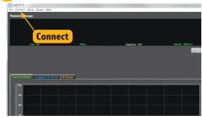
Within CygLink Software go to the menu and click "Connect" then Discover New Gauge and click "Connect". This process will likely take 10-15 seconds to find the New Gauge on the ROV. Once it is found a Notification Window will appear on screen, hit "OK". You are now ready to use the Gauge.
