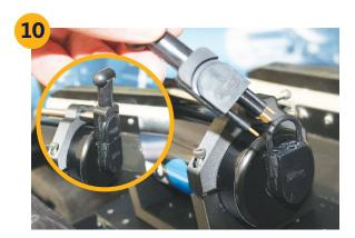
• Remove 4-Pin Blank from the rear of the Cygnus Gauge Body.
