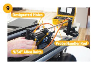
• Insert the Cygnus G1 Probe Handler Rod (B) into the designated holes on the ROV Thickness Gauge Mount Adaptor (E) as shown. With the Gimbal facing Frontwards lock the Probe Handler Rod into place using a 9/64" Allen Key.
