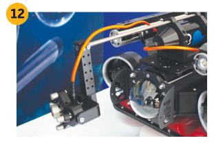
• Tidy up Wires using Wire Ties or Zip Ties and ensure the Probe has sufficient slack at the front of the ROV to allow for movement.
